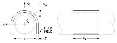
Size Range: 1/2" through 6" pipe Material: Carbon steel
